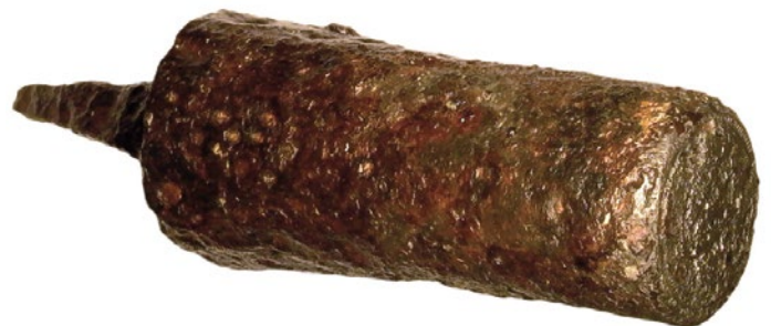
A fixed die for hammer striking anonymous coins minted by the Bishopric of Lausanne. The stamp is illegible. 14 th century.
