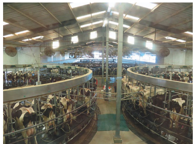
The milking parlor featuring two 48 stall rotary units, also roofed
